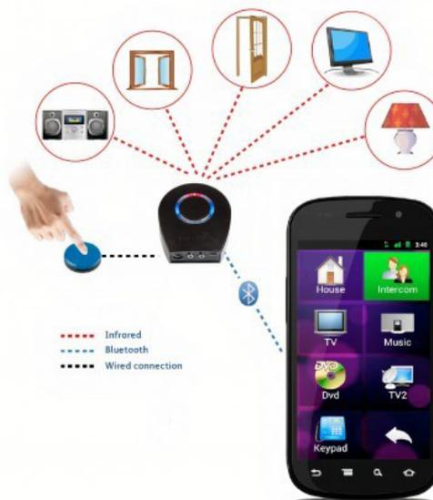
**Integration into Existing Systems:** The integration of such triggers into existing call systems is crucial. SmartLiberty offers efficient solutions, such as our “sensor modules” with jack input or the “sensor board”, which can be directly integrated into the triggers.
