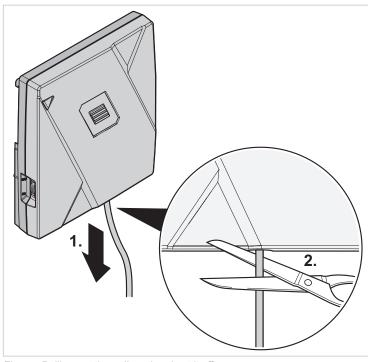
Fig. 7 Pulling out the pull cord and cut it off
