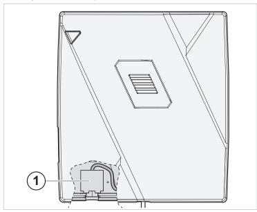
Fig. 10 Connecting the 3.5 mm mono jack plug
