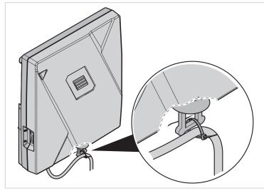
Fig. 11 Strain relief with cable tie
