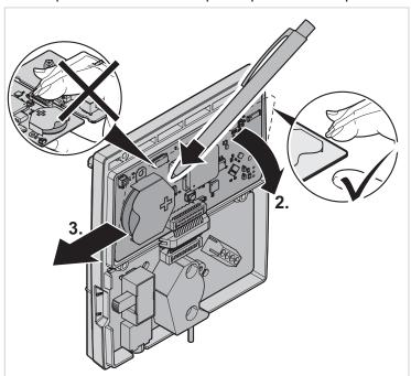
Fig. 14 Removing the battery
