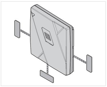
Fig. 8 Possible positions of the magnetic sensor
