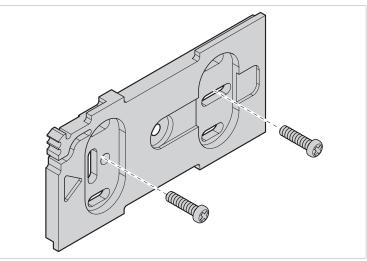
Fig. 4 Screwing the mounting plate to the wall
