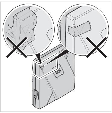
Fig. 3 Do not cover the sensor module
