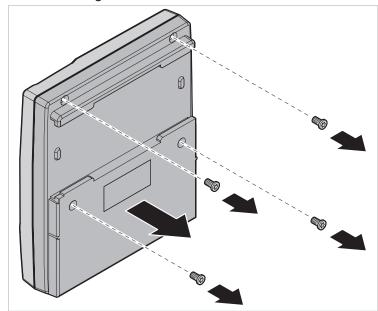
Fig. 13 Unscrewing the housing
