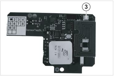
Fig. 2 Sensor board, bottom side
