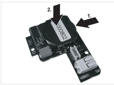
Fig. 10 Inserting the battery and sensor board
