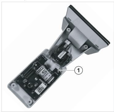
Fig. 6 Connecting the sensor board - Motion sensor
