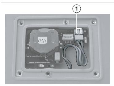
Fig. 4 Connecting sensor board - Contact mat
