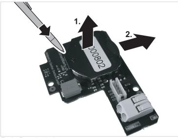
Fig. 9 Removing the battery
