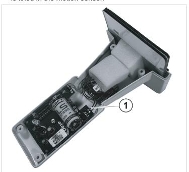
Fig. 7 Fixing the sensor board
