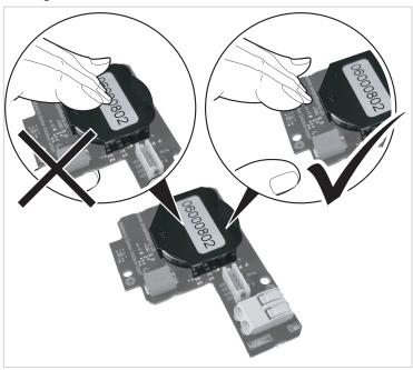
Fig. 8 Holding the sensor board by the edges
