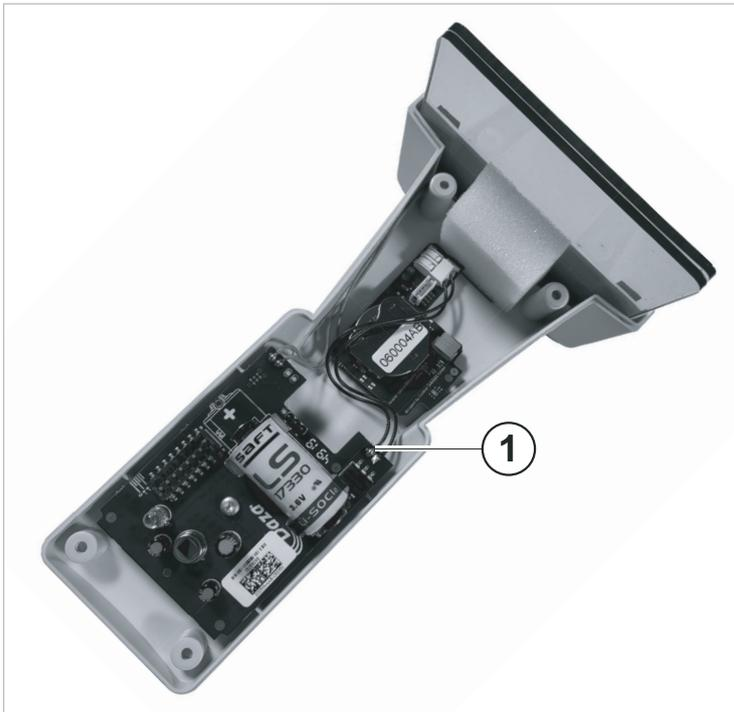
Fig. 6 Connecting the sensor board - Motion sensor
