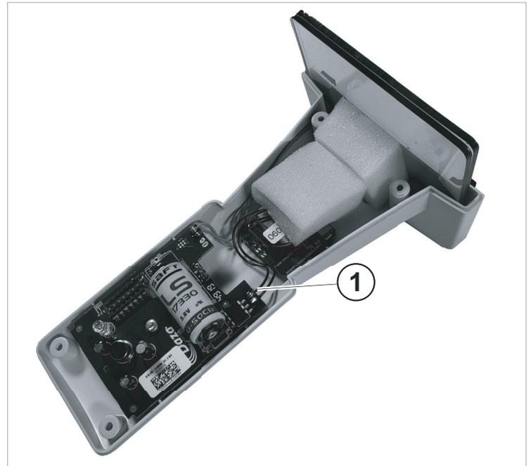
Fig. 7 Fixing the sensor board
