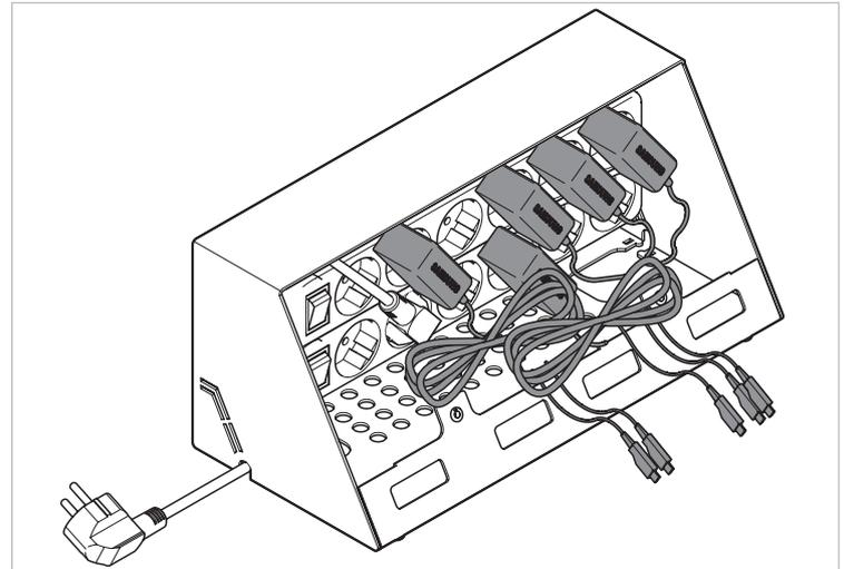
Fig. 7 Collecting the USB cable
