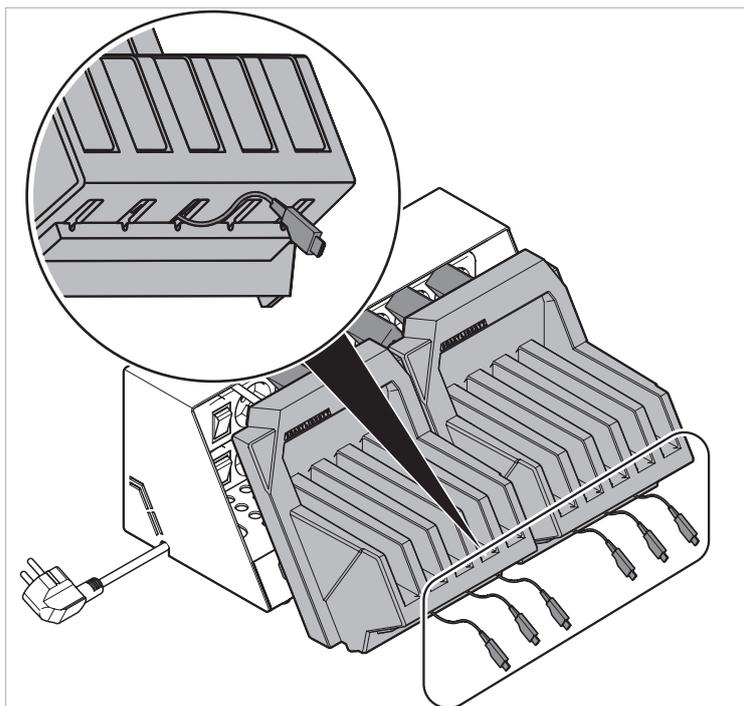
Fig. 8 Passing the USB cable through the cover
