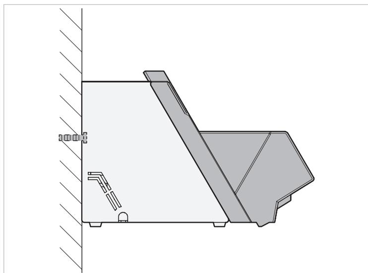
Fig. 10 Mounting the ChargerBox on the wall
