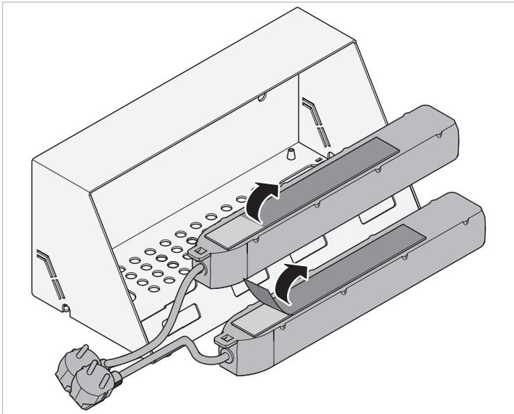
Fig. 5 Removing the protection from the adhesive tape
