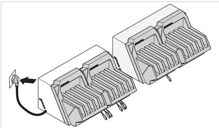
Fig. 13 Connecting the first ChargerBox
