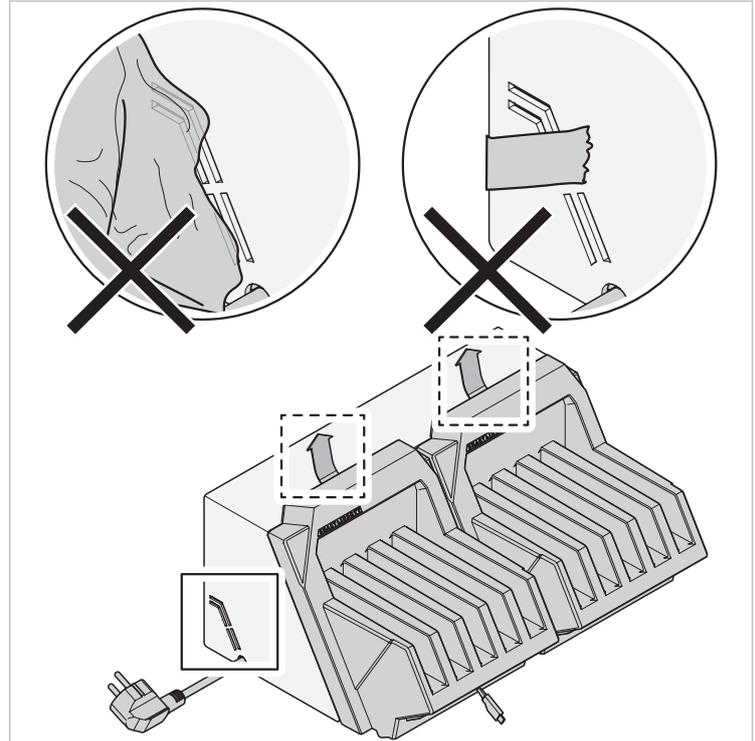
Fig. 3 Do not cover the ventilation slots (side and top)
